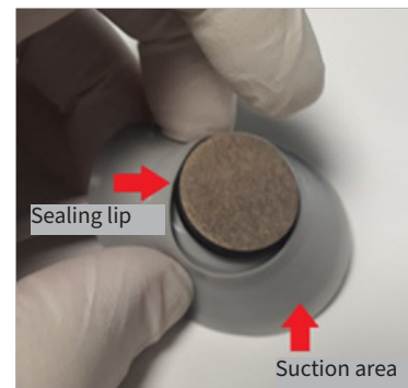
Diagram 3: Suction dome cleaning inside
