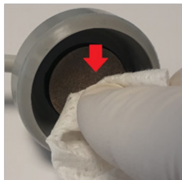
Diagram 2: Clean contact surfaces
