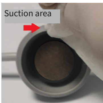
Diagram 6: Suction dome cleaning outside
