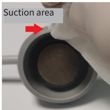
Diagram 1: Suction dome cleaning outside
