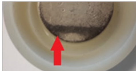
Diagram 14: Error image - discolouration of the electrode
