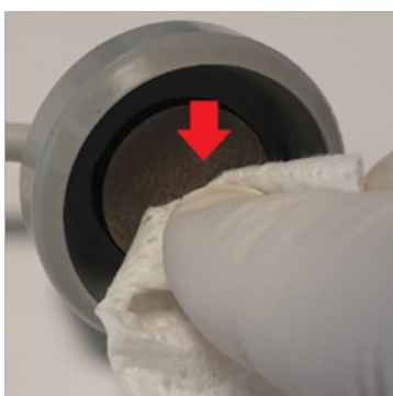
Diagram 7: Clean contact area (electrode)
