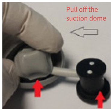
Diagram 9: Remove the suction dome
