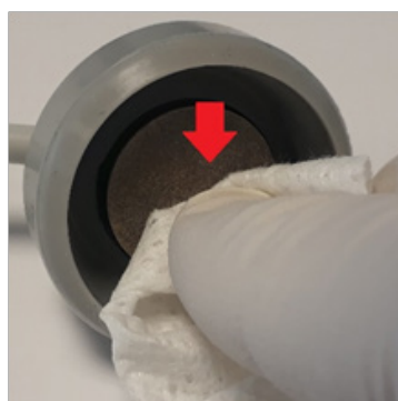
Diagram 7: Clean contact area (electrode)
