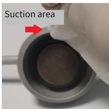
Diagram 6: Suction dome cleaning outside
