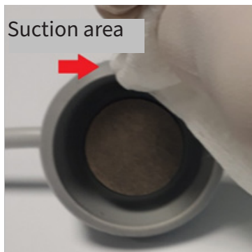
Diagram 1: Suction dome cleaning outside
