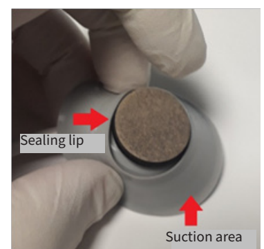
Diagram 8: Suction dome cleaning inside
