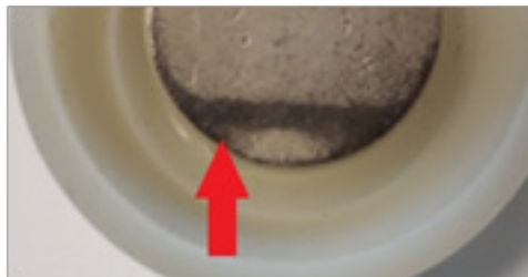
Diagram 14: Error image - discolouration of the electrode
