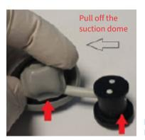
Diagram 11: Remove the suction dome
