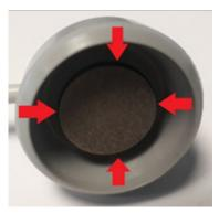
Diagram 5: Check the position of the suction dome on the electrode housing
