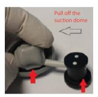
Diagram 11: Remove the suction dome
