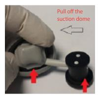
Diagram 9: Remove the suction dome
